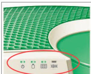
Before you start a run, check the indicator lights to ensure the instrument is ready. For information, see [Table 10](#).
